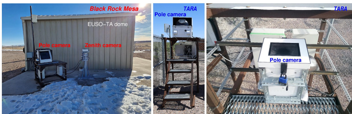
Figure 1: Installations of the DIMS cameras at the TA site. Left) Pole and zenith camera installed situated at the BRM site; Middle) Pole camera at TARA; Right) Zenith camera at TARA.
