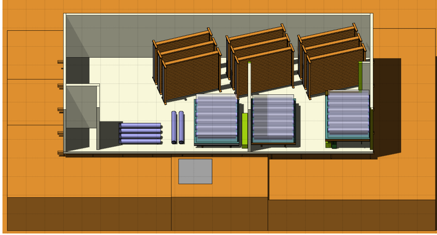
Figure 2: Geometry of neutron detectors at Mawson Station, Antarctica and their surroundings.
