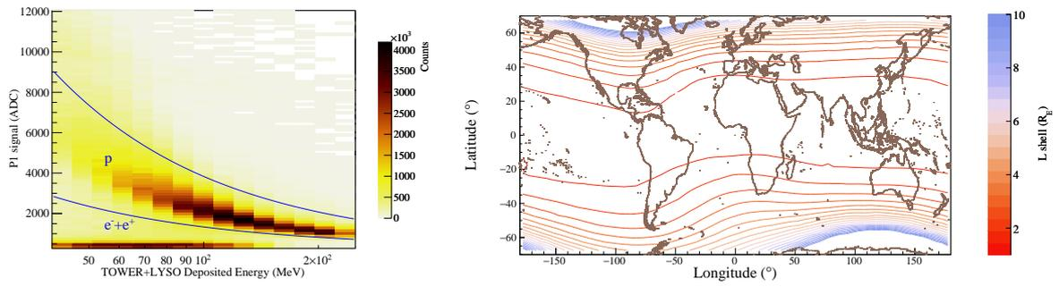
**Figure 1:** (Left) Proton and electrons+positrons signal on plane  $P_1$  as a function of the total energy deposited inside the calorimeter (TOWER+LYSO). To better visualize the separation in the plot, only vertical particles have been selected. The blue curves identify the selection employed to discriminate between protons and other populations. (Right) Map of the distribution of L shell as a function of geographic longitude and latitude, obtained using the AACGM approach.
