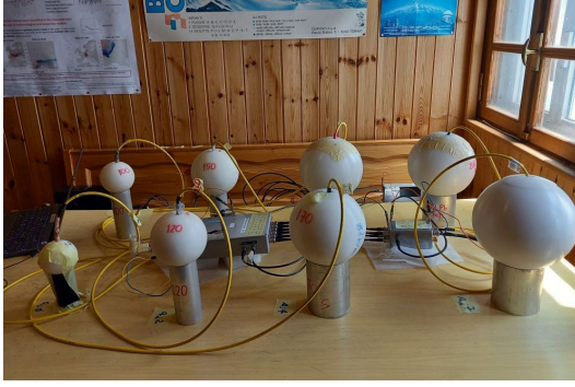
Figure 3: The S-ERBSS system composed of eight ^3\text{He} proportional counters inside six polyethylene spheres of diameter 80, 100, 120, 150, 170 and 200 mm, plus two spheres with diameter 200 mm including lead or iron inserts.
