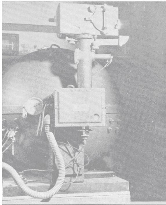
**Figure 1:** Standardized Compton-Bennett ionization chamber as operated at Huancayo.
