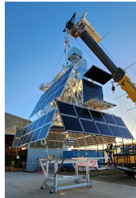
**Figure 2:** Picture from hang test before launch at Wanaka, NZ. The CT is at the front with its shutters open, and a cover to protect from sunlight while tests were done before launch.
