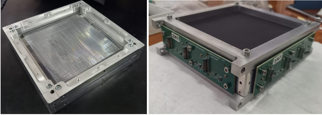
Figure 3: A FTK module without (left panel) and with (right panel) PWBs.
