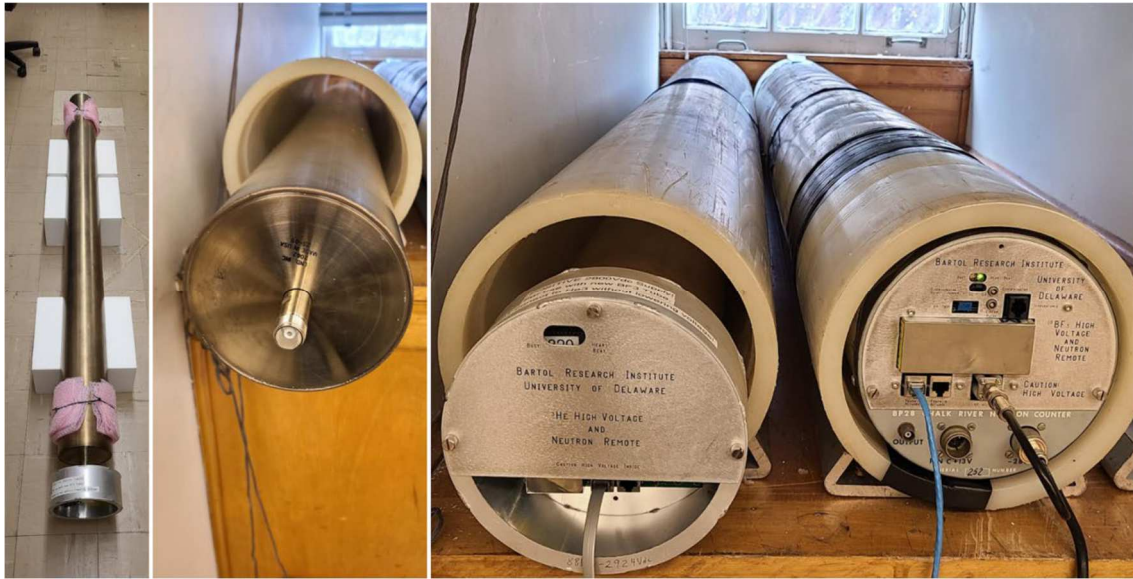
Figure 5. Photos of the LND-BP28 from Sharp Laboratory at the University of Delaware. On the right photo are shown the locations of the measurements alongside with an original BP28 [29]
