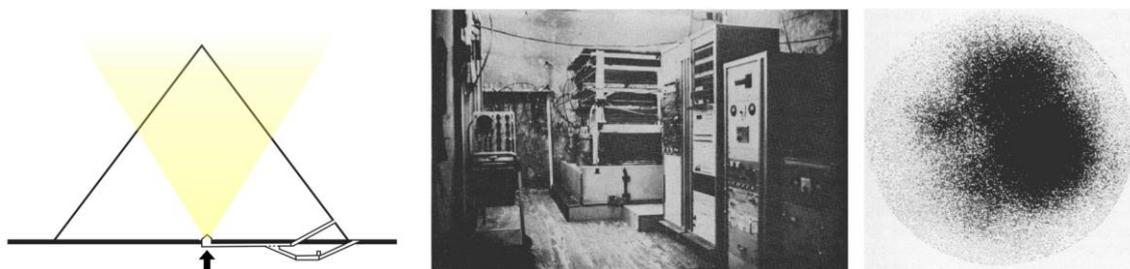
**Figure 1:** Left: A cross-section diagram of Khafre's Pyramid : the visualization range is marked with yellow areas and the Belzoni Chamber is indicated with an arrow. Center: Detector installed in the Belzoni Chamber [2]. Right: Angle distribution of detected muons [2].
