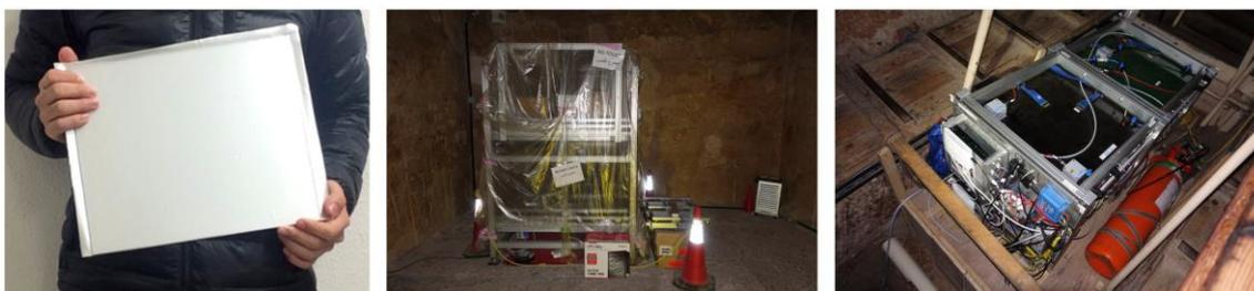
**Figure 3:** Left: A nuclear emulsion plate. Center: A scintillation detector. Right: A micro-pattern gas detector
