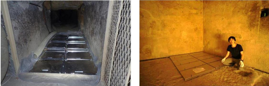
**Figure 7:** Left: nuclear emulsion detectors in the niche of the Queen's Chamber. Right: nuclear emulsion detectors placed on the floor of the Queen's Chamber [6].
