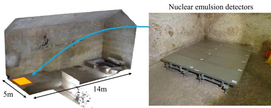
**Figure 17:** A 3D model of the Belzoni Chamber and the installed nuclear emulsion detectors. The positions of the detectors are indicated with arrows.
