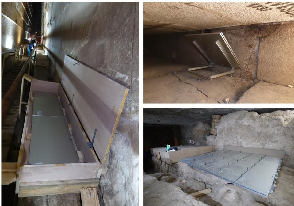
**Figure 16:** Detectors installed in Khufu's Pyramid. Left: Grand Gallery, Upper Right: Relieving Chambers, Lower Right: Subterranean Chamber.
