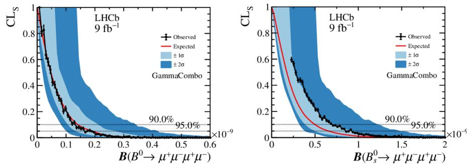
**Figure 6:** Confidence levels on the branching fractions of  $B^0$  (left), and  $B_s^0$  (right), decays to four muons.
