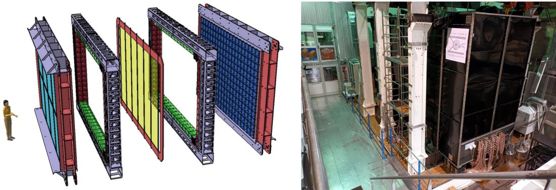
**Figure 1:** Left: An exploded view of a SuperNEMO demonstrator, showing (from left to right) one calorimeter wall, one tracker volume, the source foil, another tracker volume and another calorimeter wall [6]. Right: SuperNEMO demonstrator with antiradon tent installed.
