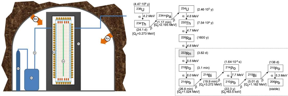
**Figure 2:** Left: Schematic view of possible Radon origins inside the SuperNEMO tracker volume. Right: Natural decay chain of the radioactive family of  $^{238}\text{U}$  [8]. One can note the presence of the gaseous Radon  $^{222}\text{Rn}$  and of  $^{214}\text{Bi}$ , which constitutes a background for the  $0\nu\beta\beta$  search.
