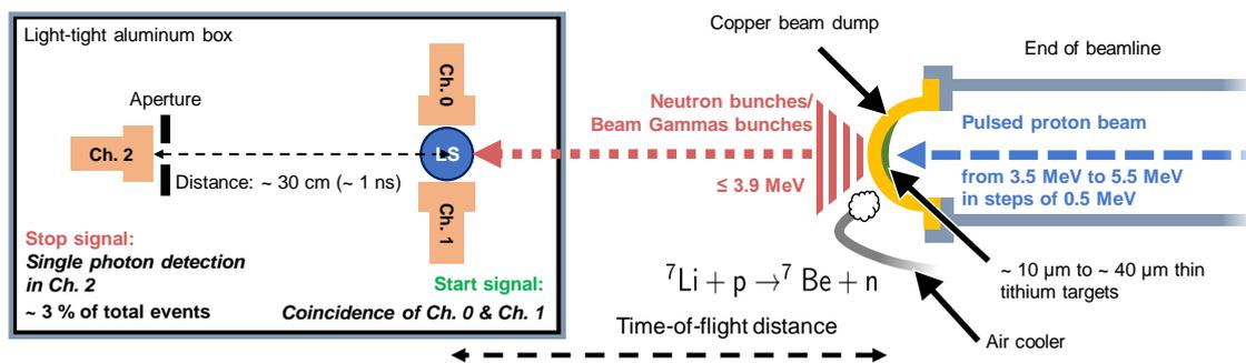
**Figure 1:** Illustration of the scintillation time profile experiment at the end of the beamline of the CN Van de Graaff accelerator at INFN Legnaro.
