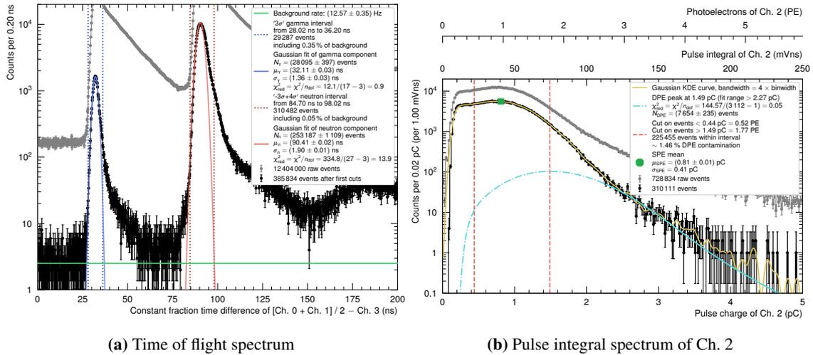
**Figure 2:** (a) Neutron and gamma data can be selected using the time-of-flight information. (b) Quality cuts on the pulse integral spectrum of the far PMT (Ch. 2) are applied to ensure single photoelectron charges.
