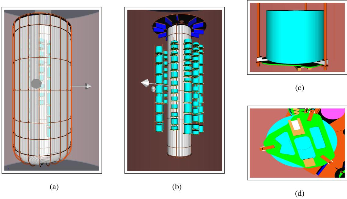
**Figure 1:** Visualization of LEGEND-200 geometry created in MaGe. (a) A complete view of the LEGEND-200 array with optical fiber shroud covering the detector strings. (b) A view of the detector strings suspended from the copper plate and the inner optical fiber shroud. (c) Side view of an individual detector unit. (d) Bottom view of a detector unit showing the PEN tile, HV and signal readout.
