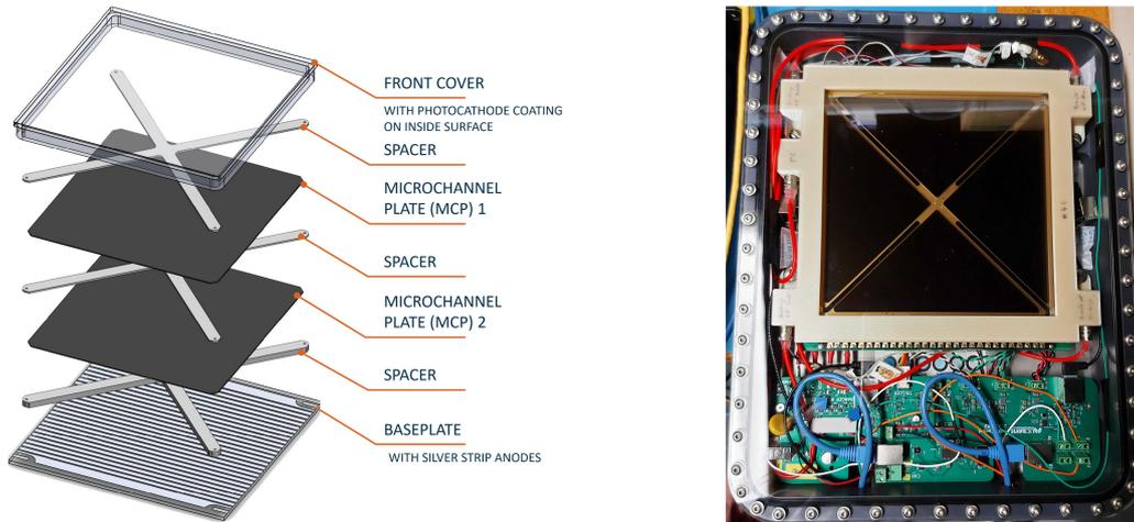
**Figure 2:** The left picture shows the LAPPD schematic setup. From the top: a borosilicate glass + cathode cover window, two levels of spacers and MCPs and a baseplate with strip line anodes at the bottom [2]. The right picture shows the complete LAPPD package as used in ANNIE. It contains the LAPPD with its mounted ADCs as well as a slow control board for sensor readout and voltage control.
