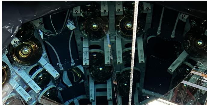
**Figure 5:** Inside view of the ANNIE tank. All deployed LAPPDs as well as some of the mounted PMTs can be seen.
