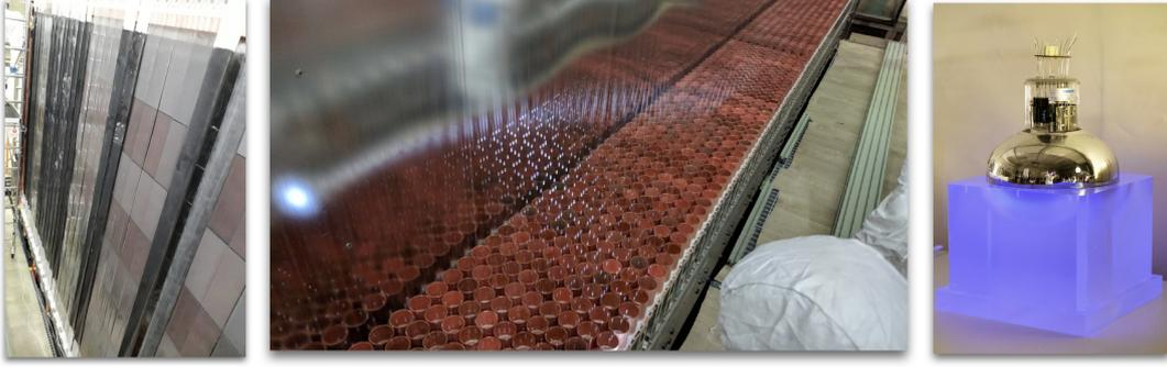
**Figure 2:** Components of the SuperNEMO detector. *Left:*  $^{82}\text{Se}$   $\beta\beta$ -decay source foils. Any solid isotope can be used. *Center:* SuperNEMO's array of 2034 Geiger cells provides 3-d particle tracking. *Right:* One of the calorimeter's 712 optical modules.
