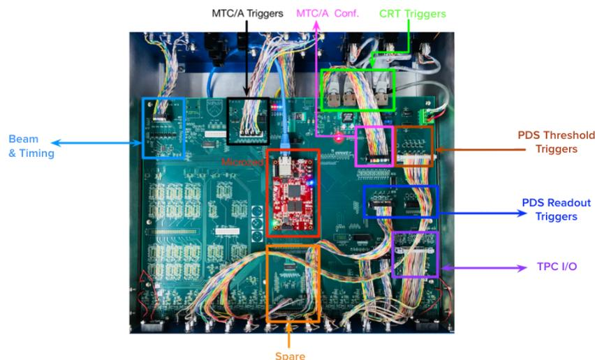
**Figure 3:** A photo of the inside of the SBND PTB enclosure, showing logic signal conversion circuitry and MicroZed in the middle. The Input/Output regions for the different SBND subsystems are labeled.
