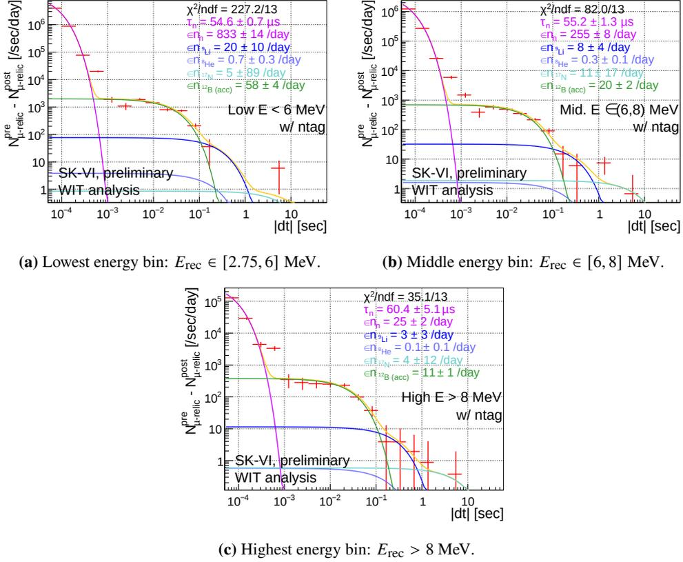
**Figure 1:** Timing distribution of spallation-like events with exponential fittings.
