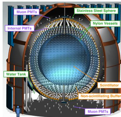
**Figure 1:** Schematic view of the Borexino detector.
