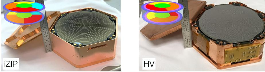
**Figure 2:** SuperCDMS SNOLAB detectors [6]. Left: iZIP. Right: HV. The iZIP detector has six phonon channels (inner core, four wedge-shaped, outer ring) and two ionization channels (inner + outer ring) on each side. The HV detector has six phonon channels (inner core, three wedge-shaped, two outer rings) on each side. The wedge channels of an iZIP (HV) detector are rotated by  $45^\circ$  ( $60^\circ$ ) with respect to the other side.
