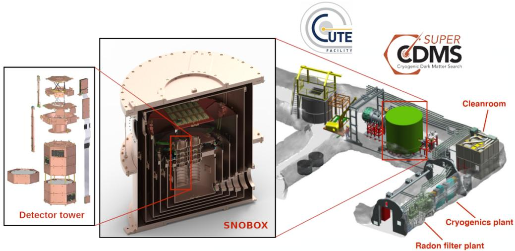
**Figure 1:** Overview of SuperCDMS SNOLAB. From left to right: Detector tower consisting of six cryogenic detectors in a copper housing; SNOBOX housing four towers; experimental infrastructure at SNOLAB including the CUTE detector testing facility, a low-radon cleanroom and the cryogenics system.
