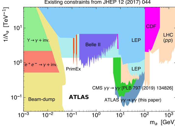
**Figure 2:** Compilation of exclusion limits at 95% CL in the ALP–photon coupling ( $1/\Lambda_a$ ) versus ALP mass ( $m_a$ ) plane obtained by different experiments. The existing limits are compared with the limits extracted from this measurement. The exclusion limits labelled "LHC (pp)" are based on pp collision data from ATLAS and CMS. [4]
