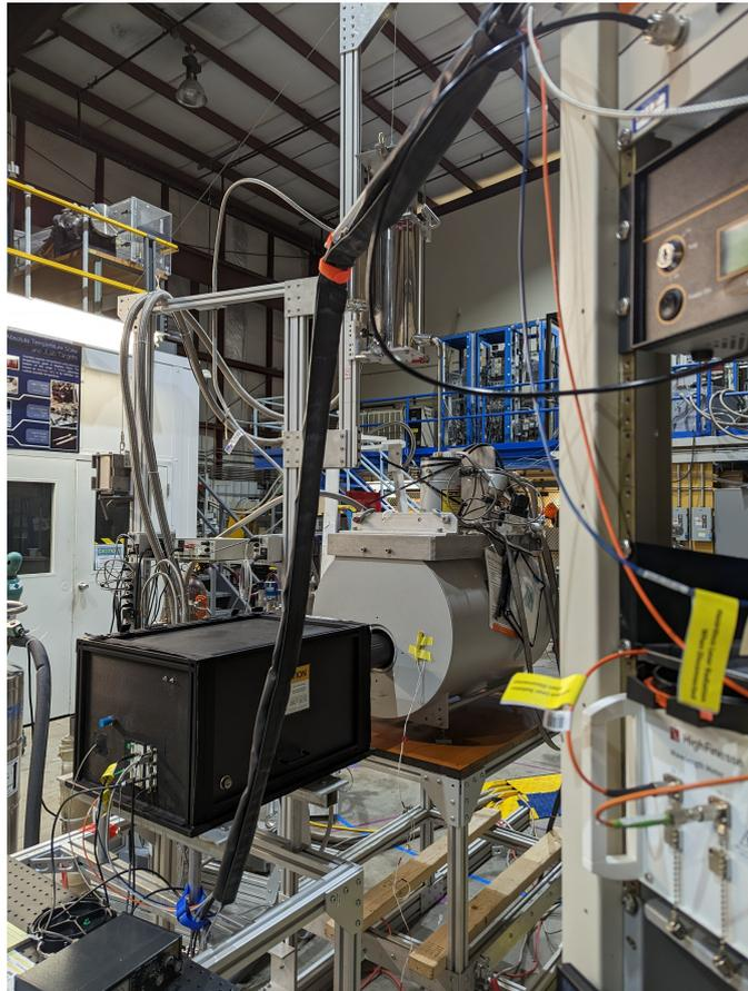
**Figure 3:** Photo of the polarization stand. The laser enclosure in black extends into the warm-bore of the superconducting solenoid to hold the pumping cell in the uniform field region.
