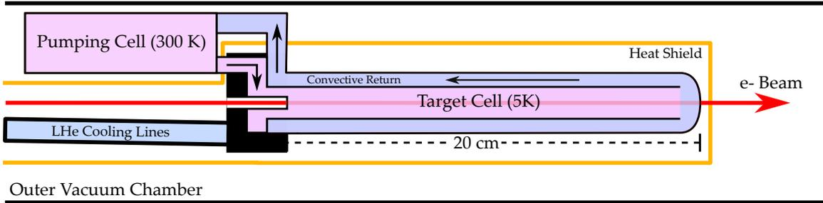
**Figure 2:** Schematic layout of the two-cell polarized  $^3\text{He}$  target concept for CLAS12.
