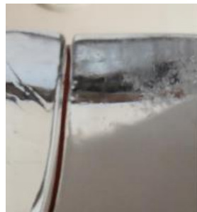
Figure 3. The hardening effect behind the wire is not observed with the thicker wire
