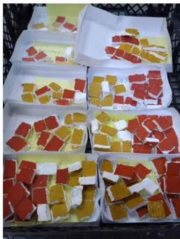
Figure 1: The mock-ups prepared under different wall painting techniques. Vermillion was used for the ones of red color, but because of their toxicity during annealing, their study was postponed.
