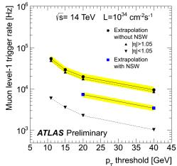
**Figure 5:** Estimation of the Run 3 L1 trigger rates, extrapolated for pp collisions at  $\sqrt{s} = 14$  TeV, as a function of the  $p_{\rm T}$  threshold [5].
