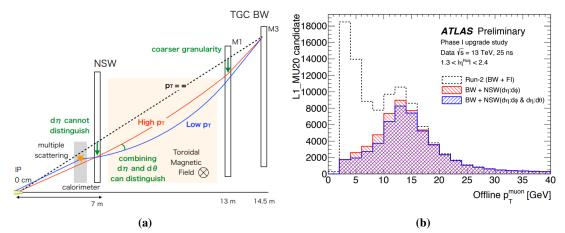
**Figure 6:** (a) Schematic diagram of the angular matching algorithm performed between the TGC Big Wheel (BW) and New Small Wheel (NSW) [4]. (b) Distribution in  $p_T$  of muons passing the L1 primary trigger, which illustrates the suppression of low- $p_T$  candidates by the TGC BW-NSW coincidence requirements [5].
