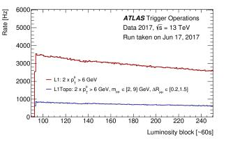
**Figure 1:** L1 trigger rate, as measured during a 2017 run, without (red) and with (blue) the L1Topo requirement. The rate is reduced by approximately a factor of 4 at the cost of a 12% reduction in the HLT efficiency with respect to offline reconstruction [3].
