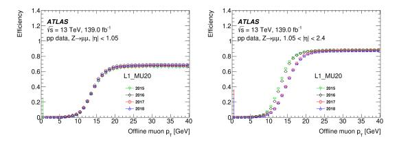
**Figure 3:** Efficiency of the L1\_MU20 trigger as a function of the offline-reconstructed muon  $p_{\rm T}$  in the barrel (left) and endcap (right) regions [3].
