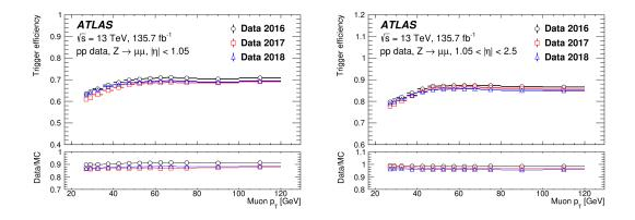
**Figure 4:** Efficiency of passing either the HLT\_MU26\_ivarmedium or the HLT\_mu50 trigger as a function of the offline-reconstructed muon  $p_T$  in the barrel (left) and endcap (right) regions [3].
