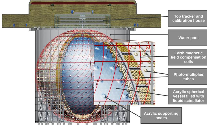
**Figure 1:** Schematic view of the JUNO detector.
