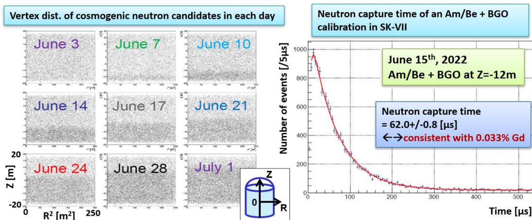
**Figure 5:** Examples of neutron monitoring in SK-Gd. The plots on the left are daily measurements of cosmogenic neutron candidate locations during the Gd addition work from SK-VI to SK-VII. The plot on the right is the neutron capture time obtained from a calibration with an Am/Be neutron source and a BGO scintillator [2] in SK-VII.
