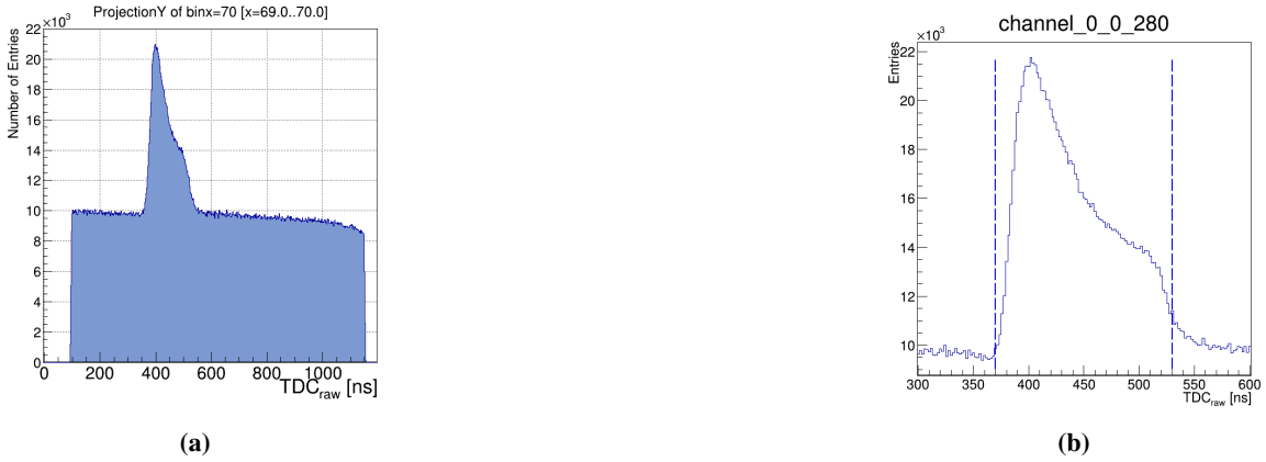
Figure 2: (a) Raw TDC time spectra of a single channel in STS1.1. (b) Expanded view in the main distribution with corresponding t_{off} and t_{max} shown by the blue-dotted lines.
