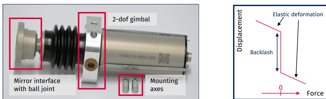
Figure 3: Left: An actuator with a 2-degree of freedom gimbal. Right: Schematic sketch of the expected force-displacement diagram in the case of only backlash and elastic deformation.
