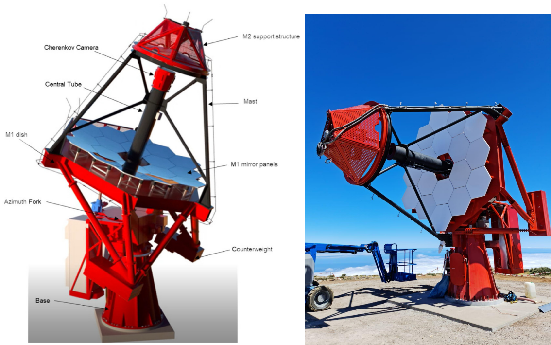
Figure 5: Left: A 3D model of an ASTRI telescope. Right: the ASTRI-1 telescope at the Teide site
