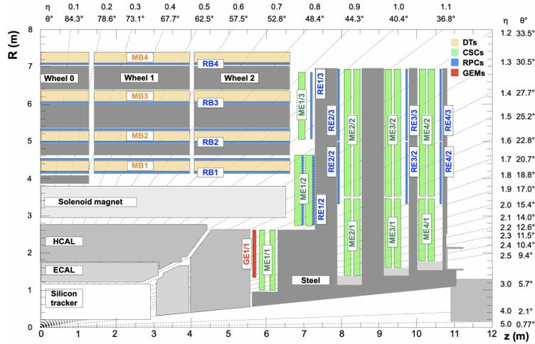
Figure 1: The CMS Muon System.
