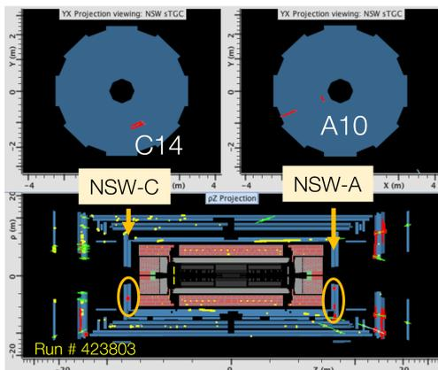
**Figure 3:** First recorded sTGC hits seen in the ATLAS event display during the special horizontal muon beam run.
