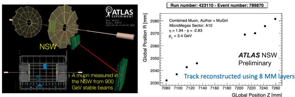
**Figure 2:** Event display of a candidate muon reconstructed by the NSW Micromegas detector during 900 GeV collision run (Left) and the corresponding track segment recorded in 8 Micromegas layers (Right).
