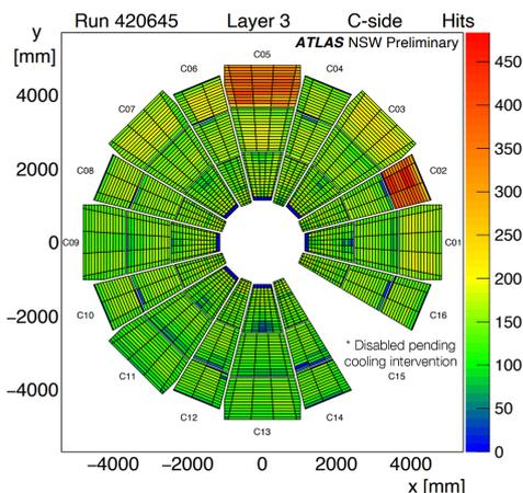
**Figure 4:** sTGC pad hit occupancy recorded by trigger electronics during the LHC beam splashes.
