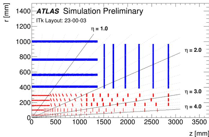
Figure 2: A schematic depiction of the most recent ITk layout. The active elements of the strip detector are shown in blue, and those of the pixel detector are shown in red. [4]
