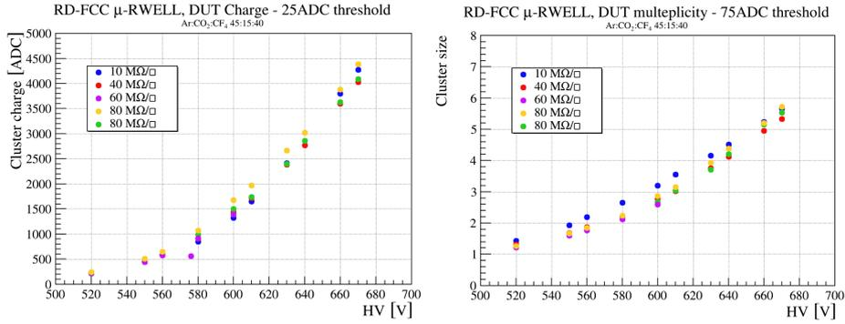
**Figure 3:** Average amount of the charge collected (left) and average number of strips fired (right) as a function of the HV on the amplification stage for different resistivity values in  $\mu$ -RWELL detectors.
