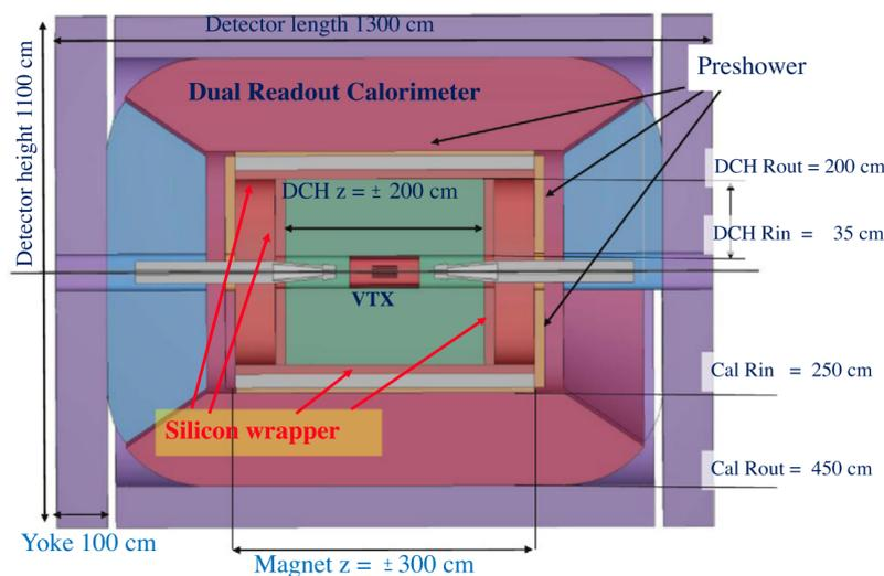
**Figure 1:** A schematic layout of the IDEA detector.
