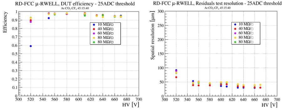
**Figure 4:** Efficiency (left) and spatial resolution (right) as a function of the HV on the amplification stage for different resistivity values in  $\mu$ -RWELL detectors.
