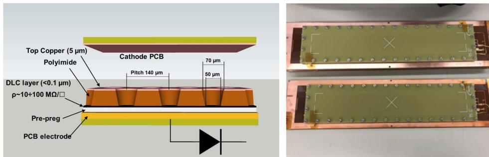
**Figure 2:** A schematic layout of the  $\mu$ -RWELL detector (left) and a picture of the detector under test in the testbeam (right) are shown.
