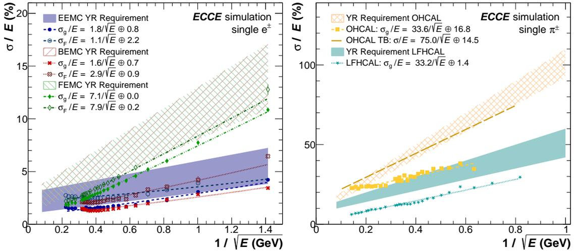
**Figure 4:** Left: Single electron energy resolution for the different electromagnetic calorimeter systems in ECCE. Right: Single charged pion energy resolution for the different hadronic calorimeter systems in ECCE. The EIC Yellow Report requirements [3] are shown as shaded bands, while full detector Geant4-based simulation data is indicated as points. Fits to the data are provided to give an estimate of the energy resolution performance.
