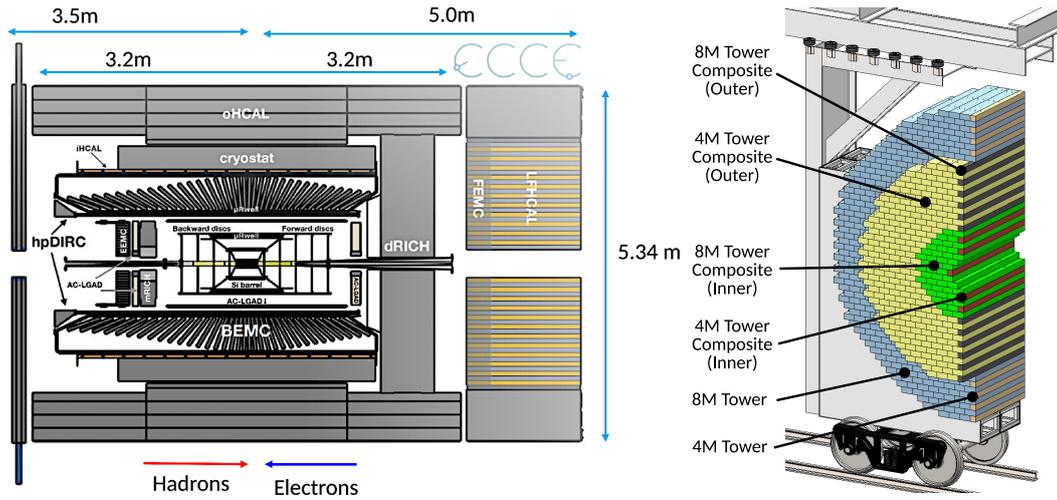
**Figure 2:** Left: Profile sketch of the ECCE detector indicating the beam directions and different subdetectors [2]. Right: Mechanical drawing of the combined FEMC and LFHCAL assembly and the various module sizes required to build the full detector geometry.
