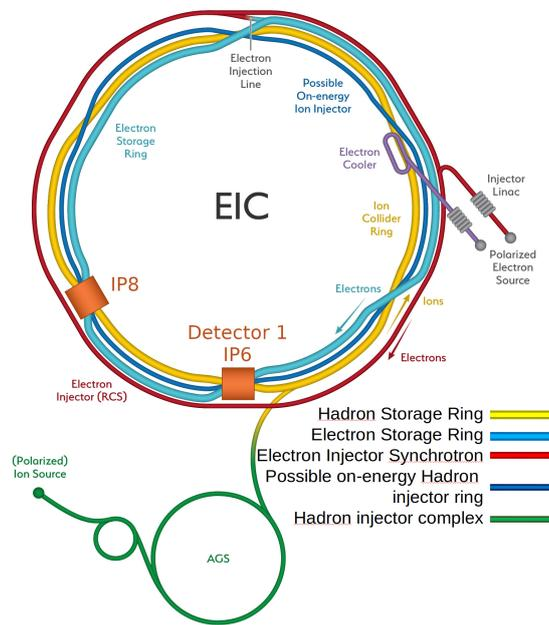
**Figure 1:** The future Electron-Ion Collider accelerator complex at Brookhaven National Laboratory including both interaction points. The hadron and electron accelerator and storage rings are shown in yellow and blue, respectively.
