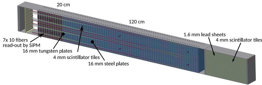
**Figure 3:** Combined FEMC and LFHCAL 8M module assembly indicating the individual components and their properties.
