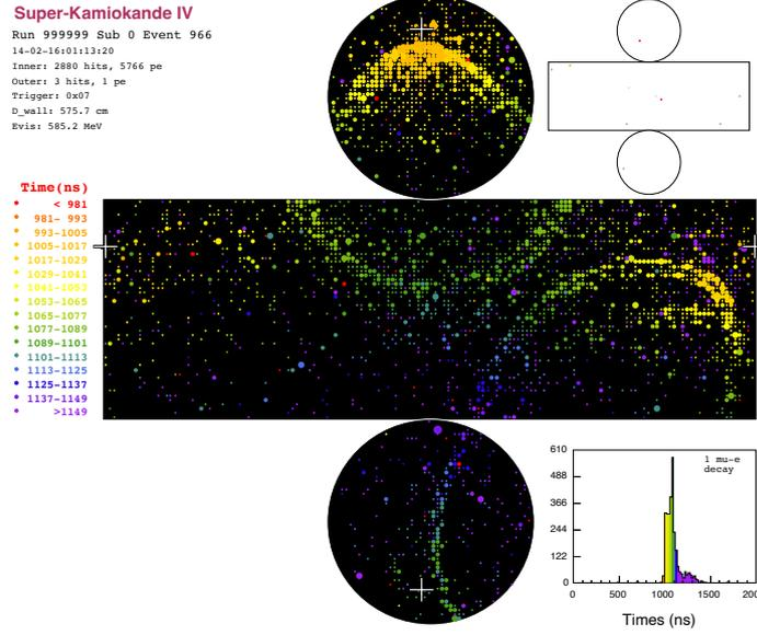
Figure 1: SK event display of a multi-ring  $\nu_e$  CC1 $\pi^+$  event, from T2K Monte Carlo simulation.
