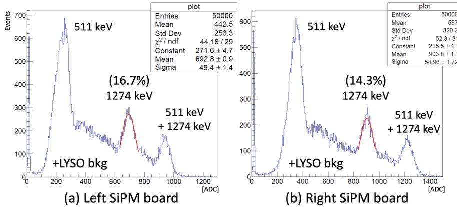
**Figure 4:**  $\gamma$  energy spectra with LYSO scintillator couple with SiPM, and customized DAQ system.
