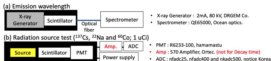
Figure 2: Experimental setup for (a) emission wavelength and (b) radiation source tests.
