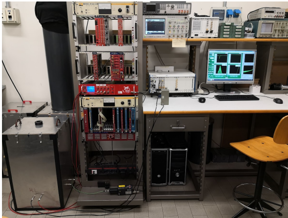
(a) Picture of the setup, including the dark box (bottom-left), power supply (center-left), digitizers (center-right) and monitor with the LabVIEW front panel (middle-right).
