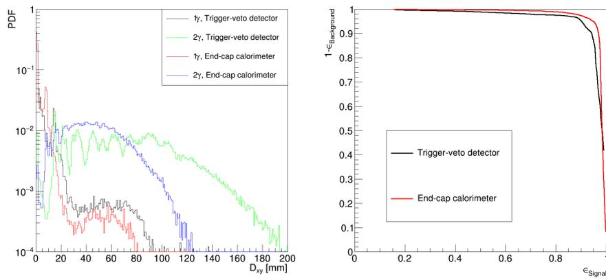
**Figure 4:** Pattern recognition distribution in the trigger-veto detector and end-cap calorimeter. (left) Receiver operating characteristic curve in the trigger-veto detector and end-cap calorimeter. (right)
