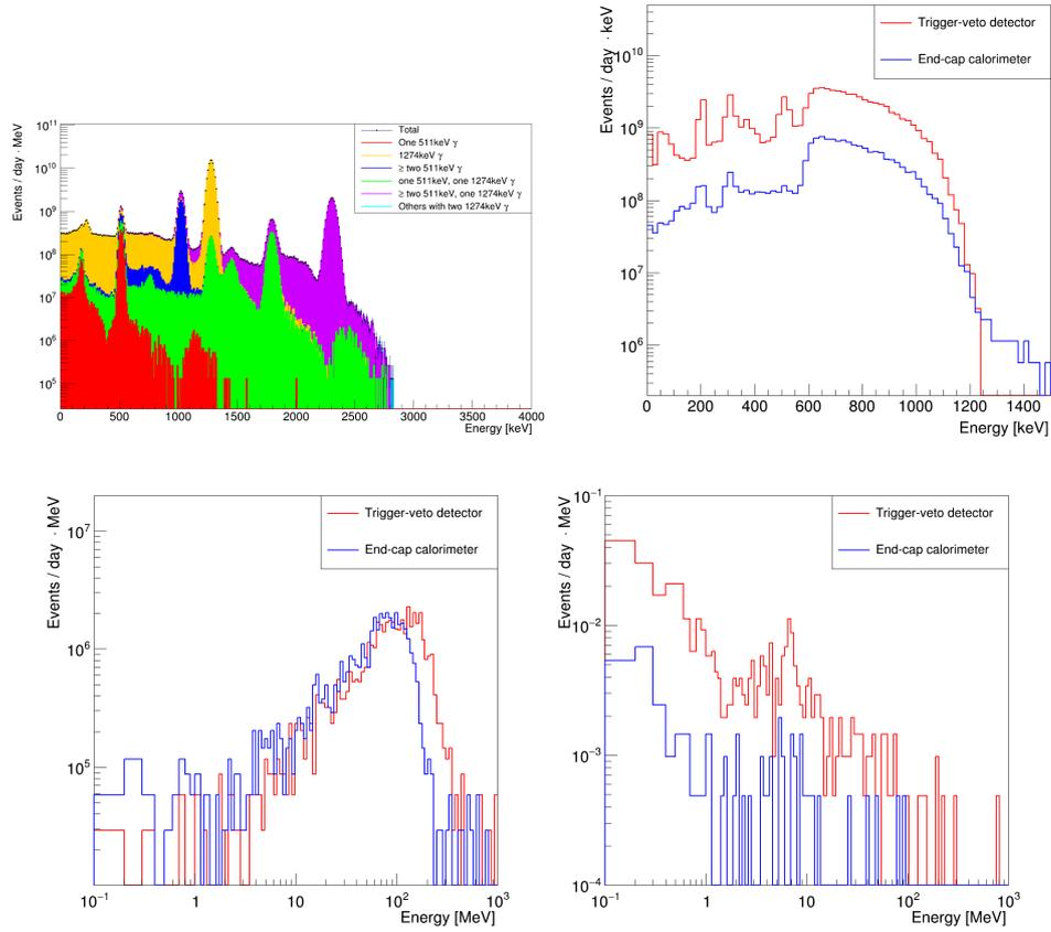
**Figure 3:**  $^{22}\text{Na}$  positron source related (top left), intrinsic radioactivity from LYSO related (top right), cosmic muons, both correlated and uncorrelated (bottom left), cosmic electromagnetic particles, both correlated and uncorrelated (bottom right)
