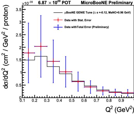
**Figure 4:** NCE differential cross-section as a function of  $Q^2$ .
