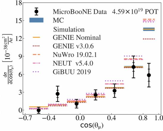
**Figure 2:** CCQE-like differential cross-section as a function of  $\cos(\theta_\mu)$ .
