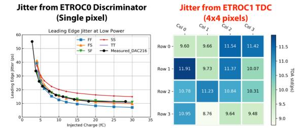
**Figure 4:** Jitter measurements from ETROC0 discriminator (left) and ETROC1 TDC (right). Taken from [14].
