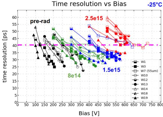
**Figure 2:** Time resolution as a function of the bias voltage of ETL LGAD sensors produced by FBK. Each color defines an irradiation fluence: (black) new sensors; (green)  $8 \cdot 10^{14} \text{ n}_{\text{eq}}/\text{cm}^2$ ; (blue)  $1.5 \cdot 10^{15} \text{ n}_{\text{eq}}/\text{cm}^2$ ; (red)  $2.5 \cdot 10^{15} \text{ n}_{\text{eq}}/\text{cm}^2$ . Taken from [7].
