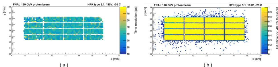
**Figure 3:** Beam test results on the time resolution (a) and hit efficiency (b) uniformity of a  $4 \times 4$  LGAD array from the HPK3.1 production. Measurements performed at the Fermilab Test Beam Facility. Taken from [8].
