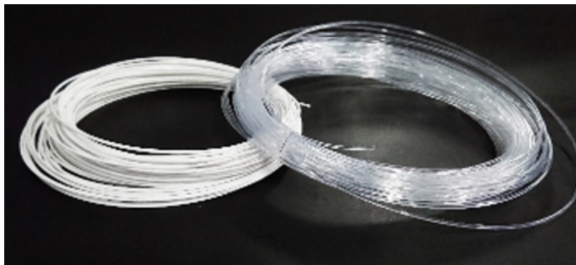
Figure 3: Scintillating and reflective filament used for 3D printing the cube matrix.
