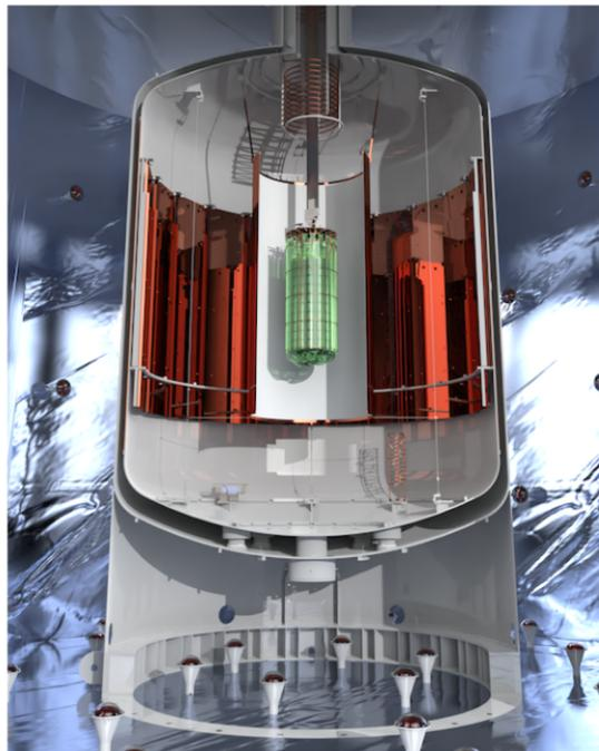
**Figure 1:** Detector systems positioned in the center of the LAr cryostat equipped with wavelength-shifting reflectors. The cryostat is placed in a water tank instrumented with photomultipliers and used as a Cherenkov muon detector.
