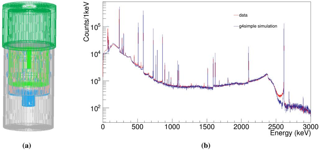
**Figure 2:** Tests on G4simple simulation. (a) Visualization of the inner components in the lead castle. (b) Comparison between data and simulation using  $^{228}\text{Th}$  source.
