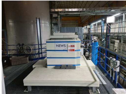
**Figure 2:** Picture of the shielded structure installed in the underground LNGS Hall C.
