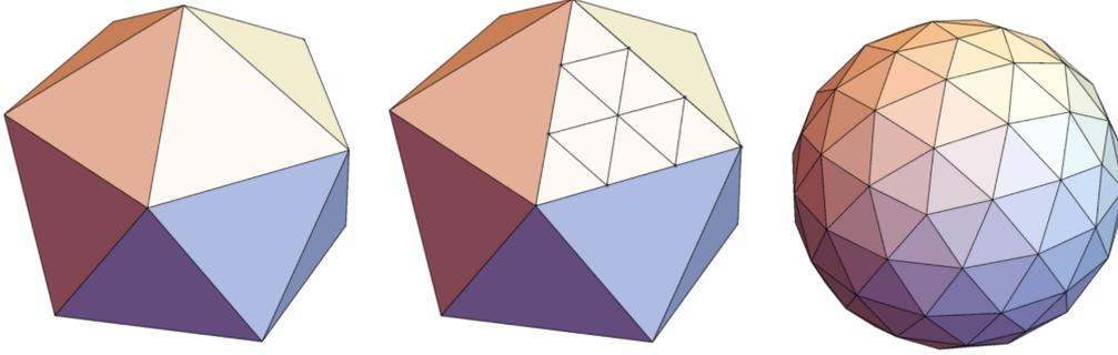
**Figure 2:** Refined icosahedron used to discretize  $S^2$ , shown for a refinement of  $L = 3$ . Each edge of the icosahedron is subdivided into  $L$  segments of equal length, which are then used to form a uniform triangular lattice on each face. The resulting points are then projected onto a unit sphere.
