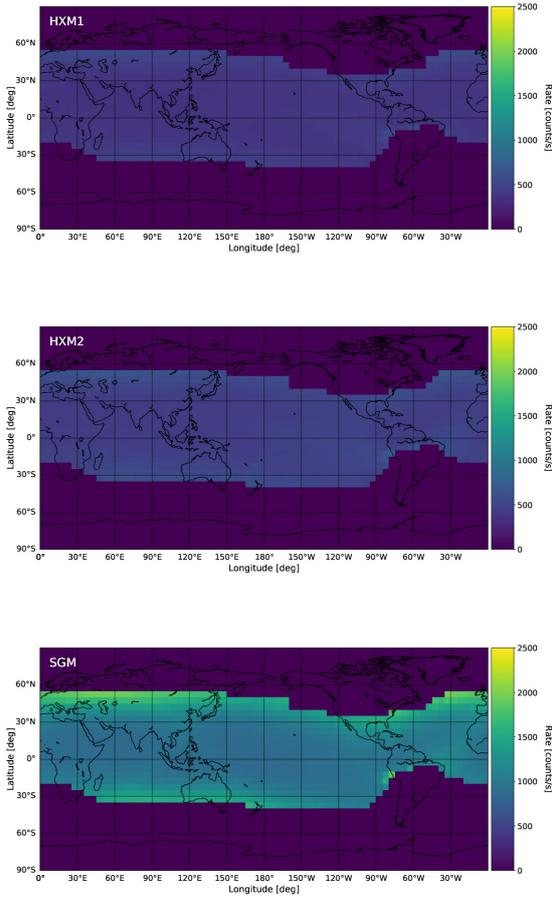
**Figure 1:** Background count rate maps measured by CGBM. The top, middle, and bottom panels are averaged count rate maps for each geographic position for HXM1, HXM2 and SGM, respectively. The count rates were calculated using PH data for September 2020 and averaged in each 5 deg. pixel.
