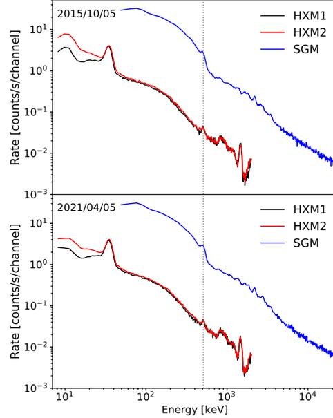
**Figure 2:** Background spectra of CGBM. The top and bottom panels show time averaged background spectra for 1000 s on October 5 2015 and April 5 2021. HXM and SGM gains were corrected by the position of 1.4 MeV and 2.2 MeV lines for each. Gray dotted lines show the position of 511 keV.
