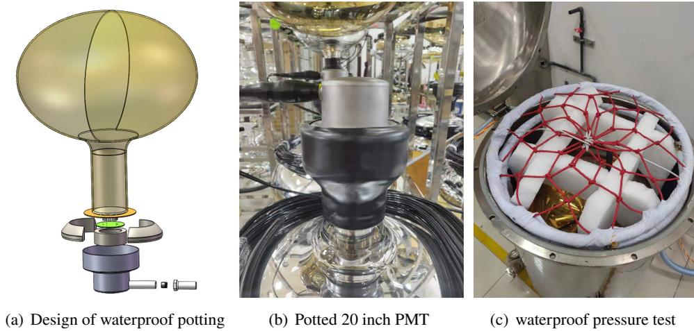
Figure 4: Details of PMT potting.
