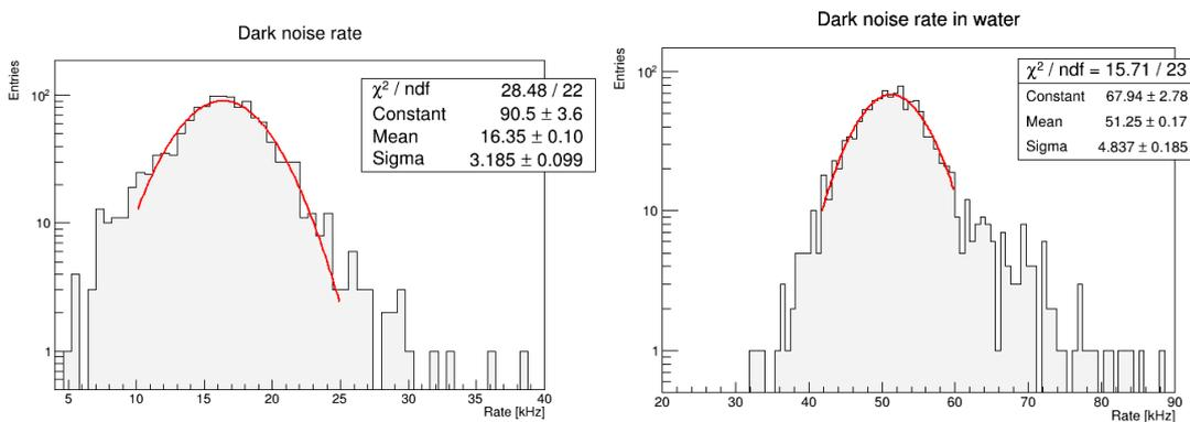
**Figure 3:** Left: dark noise rate without water, Right: dark noise rate in 4.5 meters of water.
