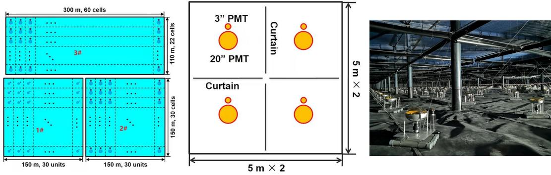
**Figure 1:** Schematic of LHAASO-WCDA. Left: full picture of the LHAASO WCDA, where are shown the three pools. Middle: Scheme of the arrangement of the PMTs in WCDA-3. Right: a picture of the inside of WCDA-3.
