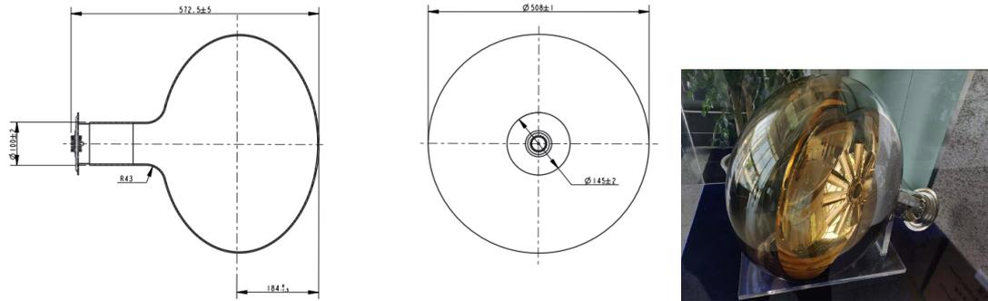
**Figure 2:** Dimension of 20 inch MCP-PMT.
