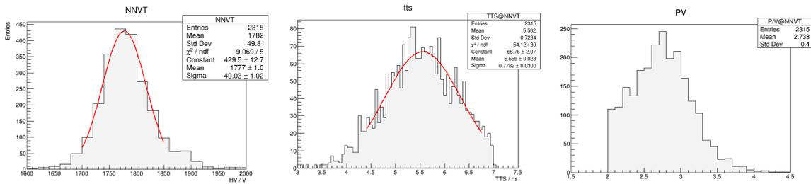
**Figure 6:** Part of test result at NNVT. Left: the distribution of working voltage, Middle: transit time spread, Right: peak-to-Valley ratio.
