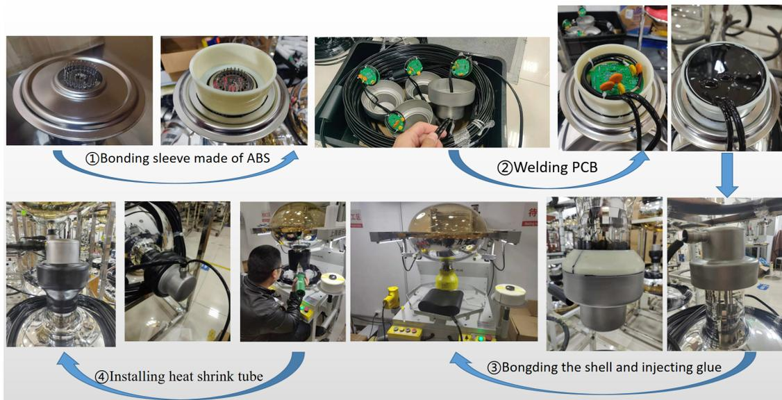
Figure 5: PMT potting procedure
