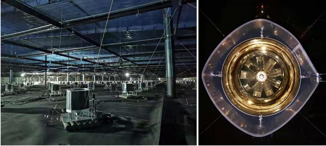
**Figure 7:** Left: full view of magnetic shield-Permalloy installed on 20 inch MCP-PMT. Right: top view of PMT.
