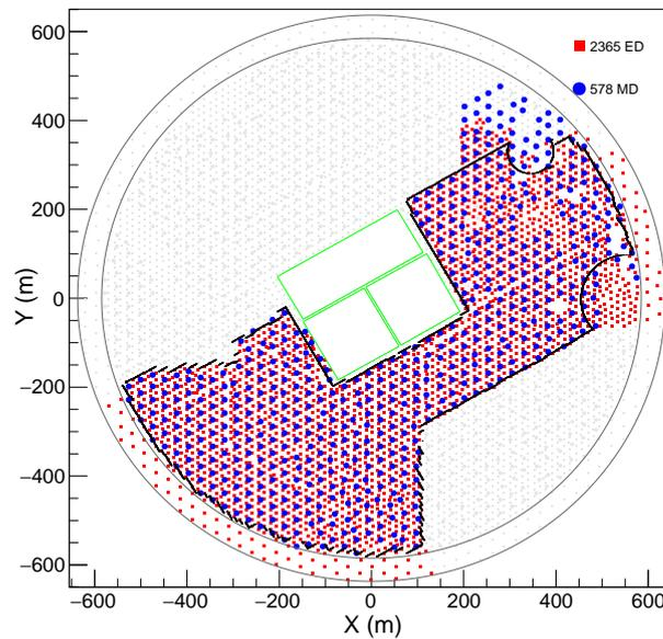
**Figure 1:** Planned layout of all LHAASO-KM2A detectors. The red squares and blue circles indicate the EDs and MDs in operation, respectively. The area enclosed by the dotted black line outlines the fiducial area of the current KM2A half-array used in this analysis. The central green squares indicate the LHAASO-WCDA array region.
