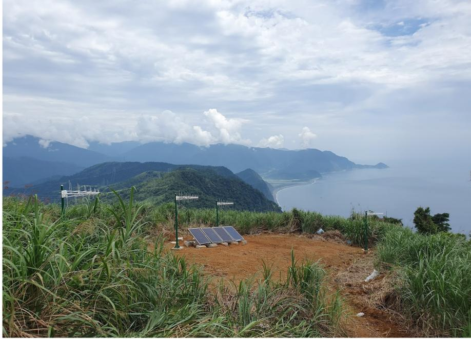
**Figure 2:** TAROGÉ-4 station, LPDA antennas pointing horizontally to ocean.
