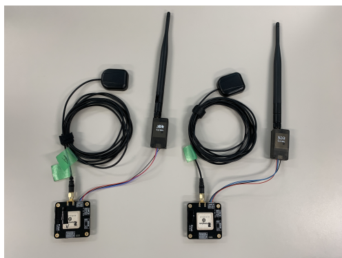
Figure 3: The Piksi is composed of two modules and records the relative position of them.
