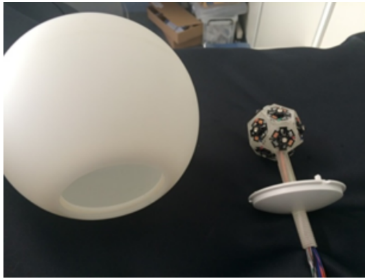
Figure 7: The light source mounted on the Opt-copter is consisted of 12 UV-LEDs attached on dodecahedron and a spherical diffuser.
