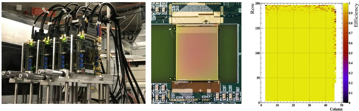
**Figure 2:** The MuPix Telescope (left) and MuPix8 chip (middle) used for the test-beam at PSI with the resultant measured hit efficiency of the sensor (right).
